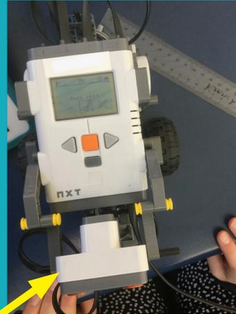
We moved the ultrasonic sensor to the side because the robot was too long to turn well and was 5 cm over the length allowed in the rules.
